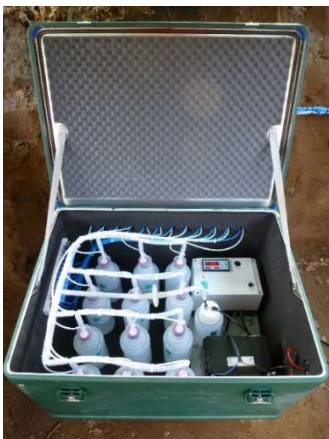
Aluminium box with electronic vacuum control, power supply and collection bottles for the suction plate system
