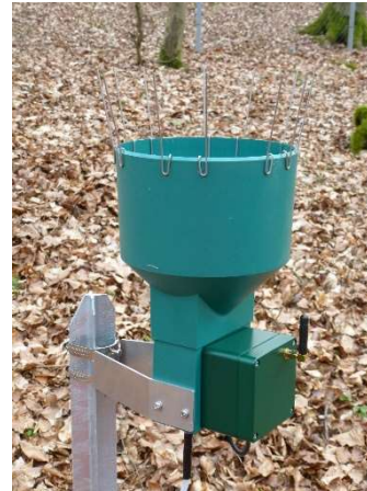
Tipping bucket rain gauge with remote radio logger
