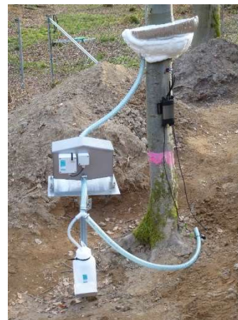
Pre-assembled system for recording the stem flow
